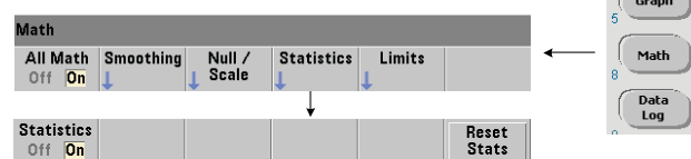
FIGURE 3: Enabling statistics from the front panel
